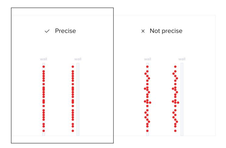
A precise point cloud, as shown on the left, has little "noise" - the points closely match the shape of the real-world object
