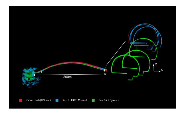
This is the sewer cross section at the end of the flight. As you can see, the green Rev 6.2 has significantly more drift, reaching 1.4%, compared to the Surveying Payload Rev 7 and FARO Connect, which only has 0.19% drift.
