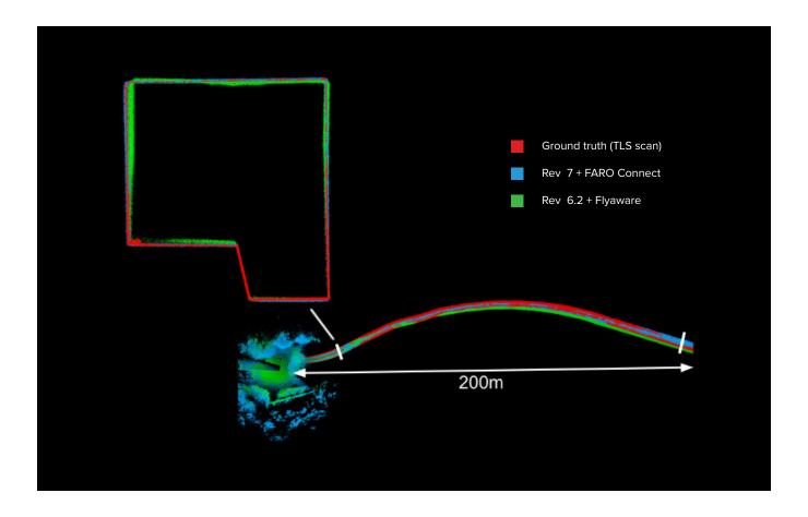
This cross-section from the beginning of the tunnel shows colored point clouds from the LiDAR Surveying Payload (Rev 7), the Terrestrial Laser Scanner as a control dataset, and the standard Elios 3 LiDAR, the Rev 6.2. This was the area used to align the different point clouds with the ICP settings in FARO Connect.
