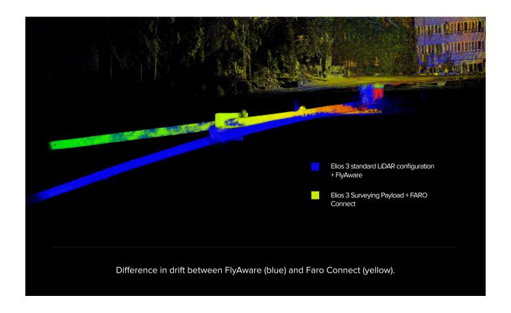
With greater geometrical features in a similar environment, it may be possible to reduce the drift. However, considering the challenge of this location, the Surveying Payload's Rev 7 handled the survey very well with better results than the Rev 6.2.
