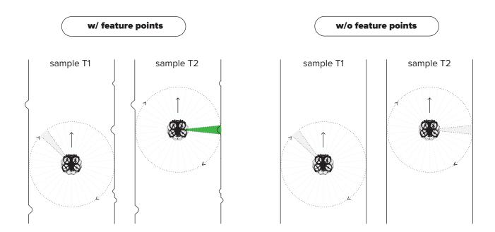
When there are fewer geometric features, as in highly symmetrical environments, it is harder for the LiDAR to detect key features of reference that enable it to correctly interpret its surroundings, causing it to accumulate drift
