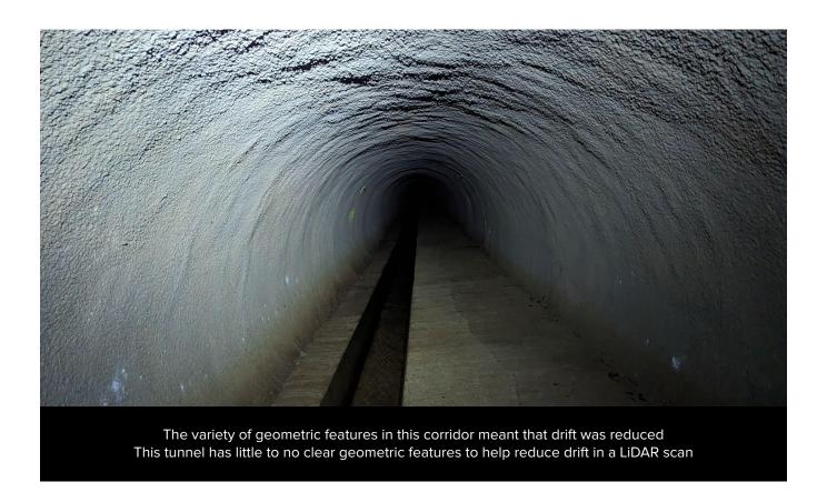
In this testing environment, the Rev 7 payload was compared to the Rev 6.2 in a sewer with greater than 2 meter diameter. The only geometric features were walkways, a gully, and shotcrete with textured surfaces.
