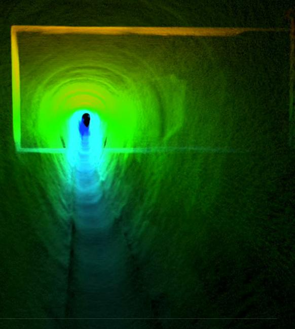
As part of final testing, the Rev 7 Surveying Payload was then used to scan another sewer environment. It was considered to be very challenging because the diameter was less than 2 meters (0.8m to be exact). In addition, there were few geometric features or textures in straight sections.
