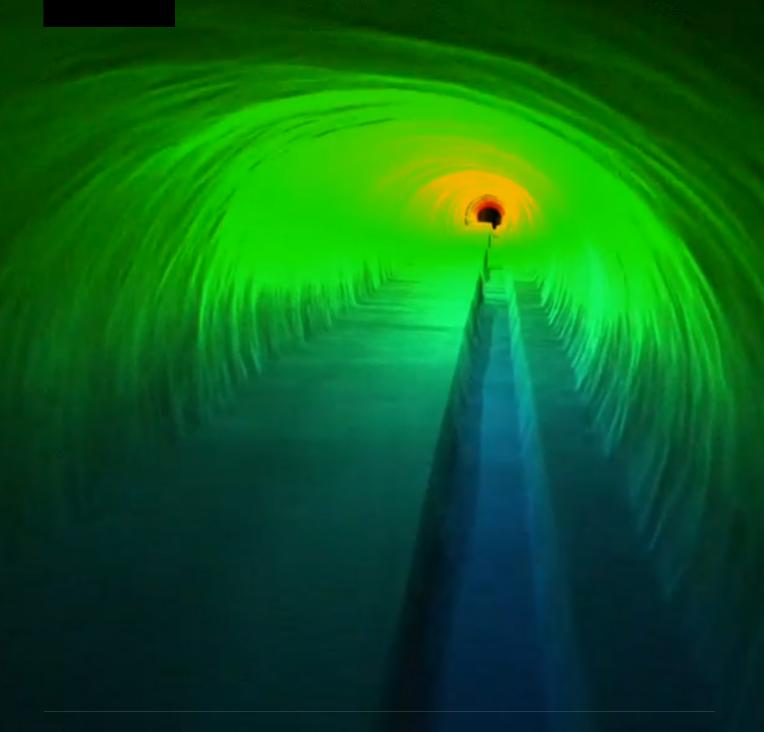
The Surveying payload was tested in increasingly challenging environments. A challenging symmetrical environment is one with light geometric features or texture in prolonged straight areas (greater than 30-50 meters), as well as a diameter greater than 2 meters. Examples of environments with these features could include tunnels, stacks, and shafts.
